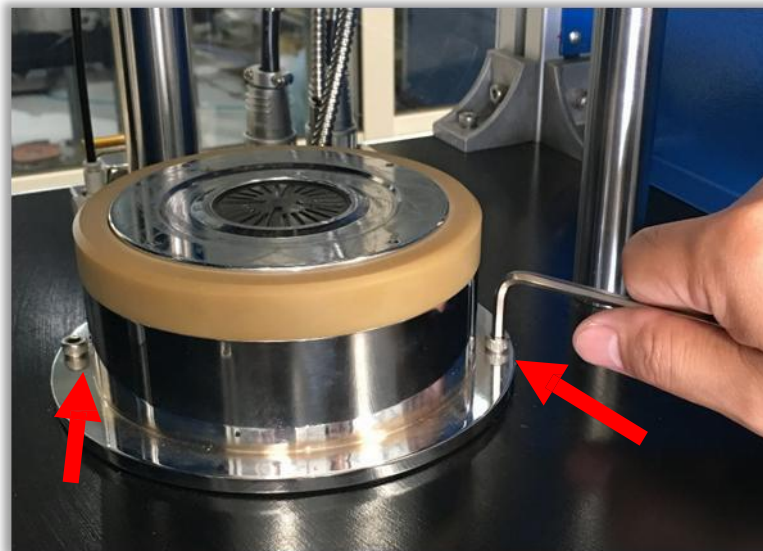
Figure 42 shows removal Cover from the Lower Die by remove 2 screws
