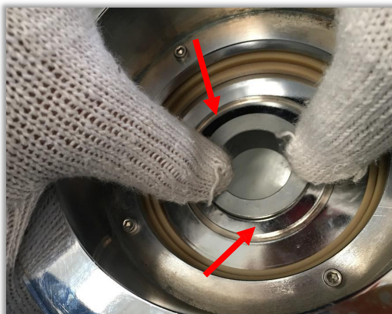
Figure 47 shows using Jig for supporting O-ring replacement
