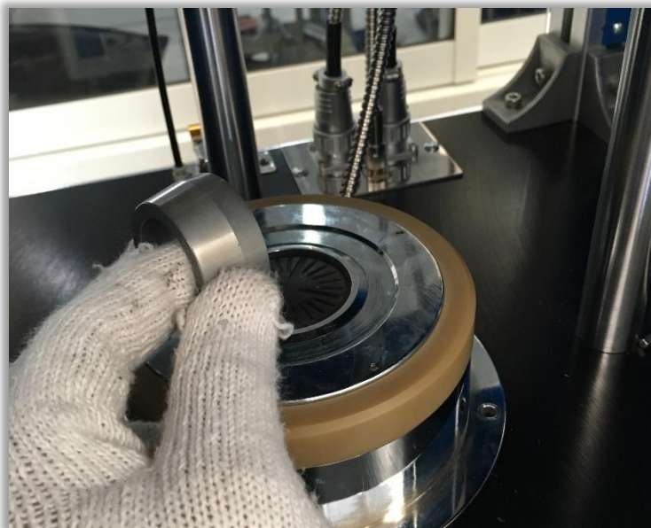
Figure 49 shows removal Jig from O-ring
