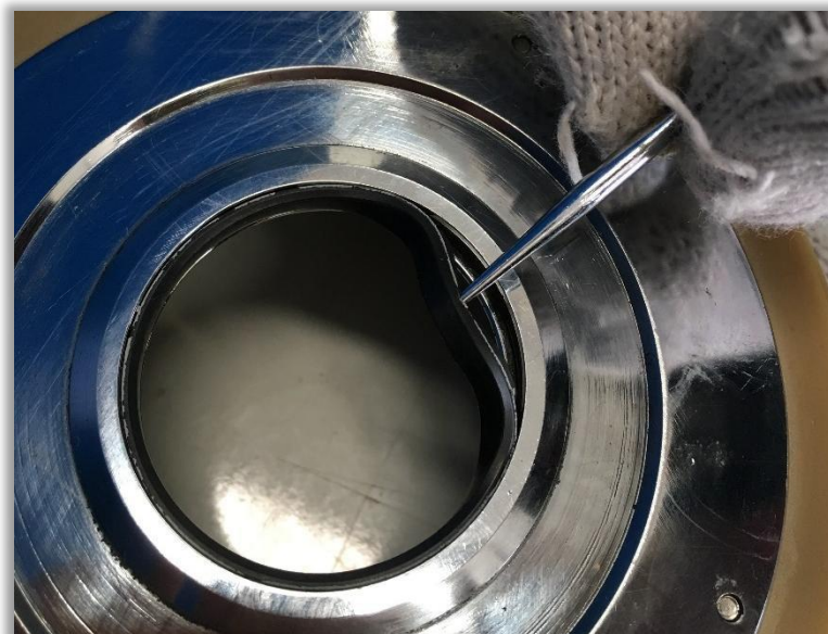
Figure 45 shows replacement the old O-ring from Cover of the lower die
