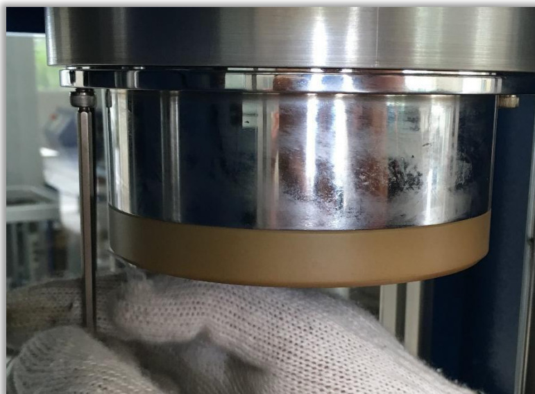
Figure 50 shows removal Cover from the Upper Die by remove screws.
