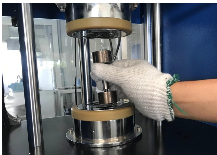
Figure 41 shows how to move Torque Standard out of MDR-01
